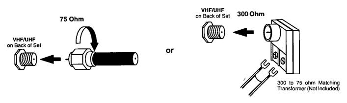
Cable Connection – For reception of cable channels, connect the cable supplied by your local cable company. In the SETUP menu, set the MODE to CABLE. (Refer to Antenna Mode section.)
